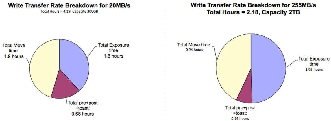
Figure 1: Write transfer rate breakdown illustrating major contributors to write transfer speeds
