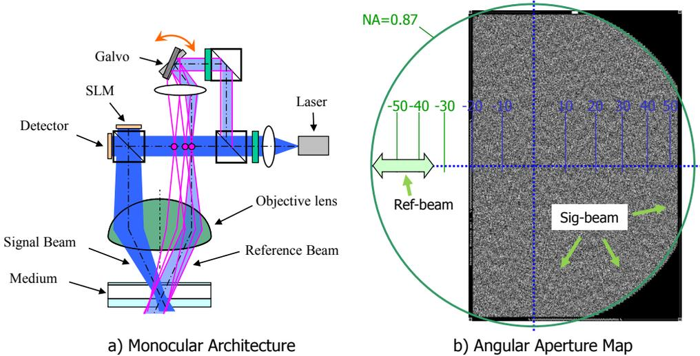
Figure 2: a) Monocular recording System. b) Monocular system angular aperture map
