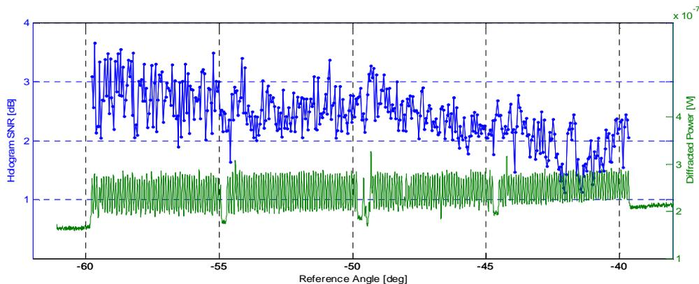
Figure 7. SNR and diffracted power of holograms recovered at an areal density of 2 Tbit/in<sup>2</sup>.
