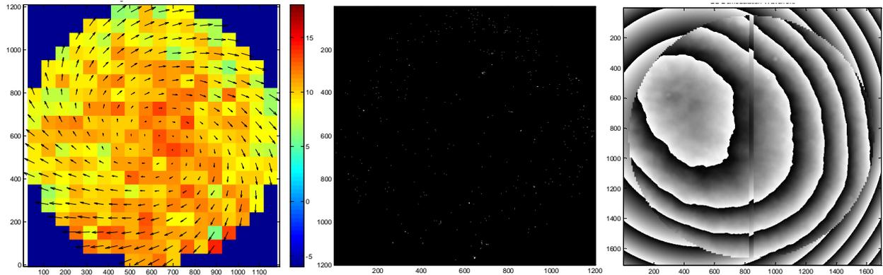
Figure 5. SNR map, BER map, and homodyne wavefront for a BPSK hologram recorded at density on the Tapestry drive.
