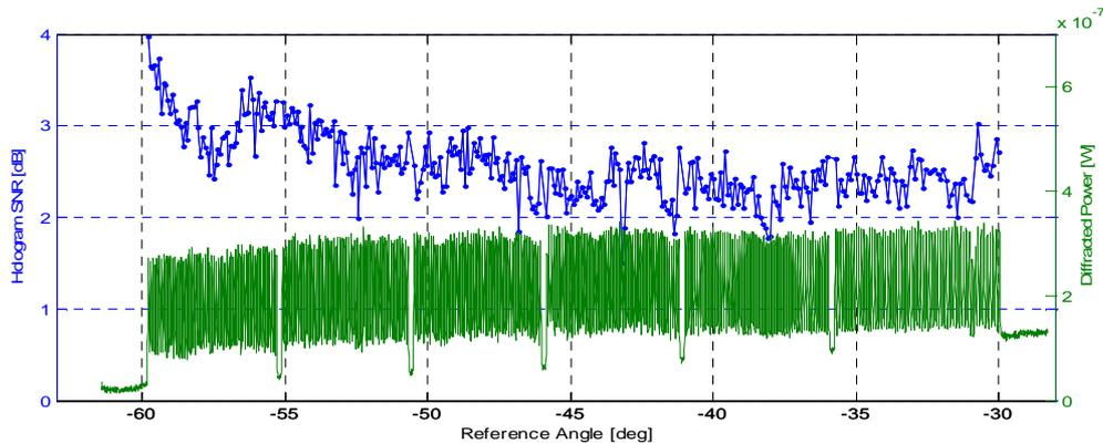
Figure 4. SNR and diffracted power of holograms recovered at an areal density of 1.53 Tbit/in<sup>2</sup>.
