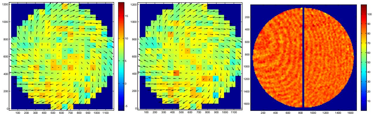
Figure 6. SNR maps for I and Q QPSK holograms and phase difference map.
